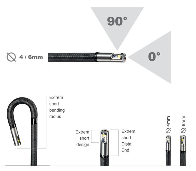
Dual vision starting at a diameter of 4mm. The side mounted 90° camera is directly mounted at the distal end. Therefor you have dual view direct and without delay. The distal end is through its extremely short design capable of the best possible navigation properties and a small deflection radius.
